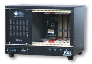
4-slot PXI chassis, 4U high, 3 I/O slots, forced-air cooling with 90-cfm fan, front-mounted power switch, 275W power supply, 10x7x8.25 inches (W x H x D)
